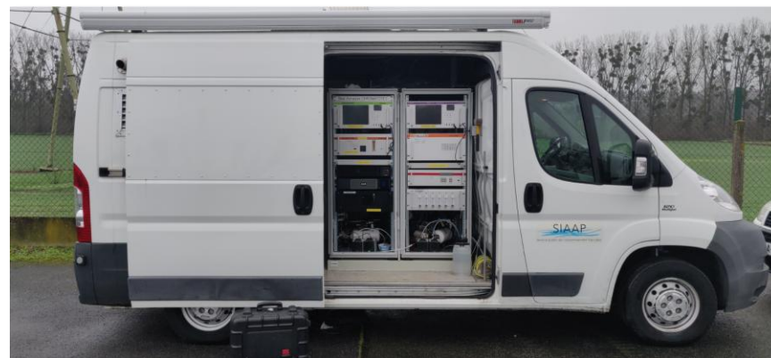
Emergency mobile van for waste water treatment plant in Paris with VOCs and sulfurs
