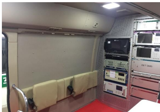
Emergency mobile van for industrial area with full airmOzone MS
